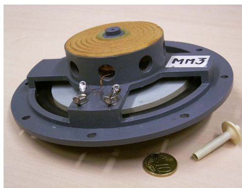
FIG. 5. (Color online) Picture of the prototype driver (MM3c) with a 10 Euro cents coin. At the position where a normal loudspeaker has its heavy and expensive magnet, the prototype driver has an almost empty cavity; only a small moving magnet is necessary, which is shown in the right corner.
